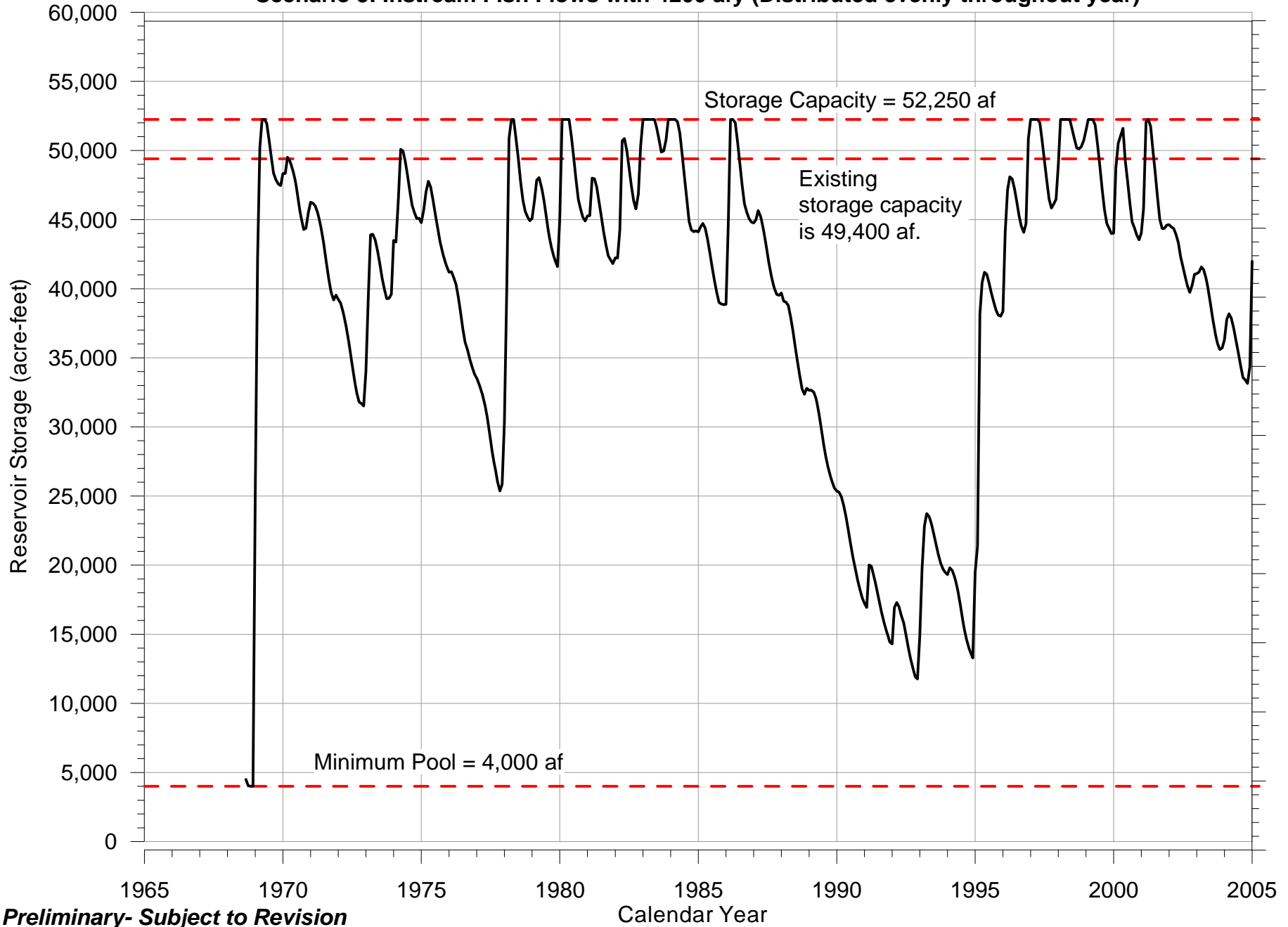
Figure 3. Simulated Lopez Reservoir Storage Assuming 3'-Raise Scenario 3: Instream Fish Flows with 4200 afy (Distributed evenly throughout year)
